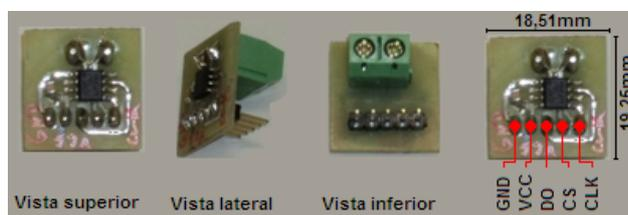
**Figura 5.** Placa do MAX6675, onde GND = *Ground*, VCC = *Common-collector voltage*, DO = *Data out*, CS = *Chip select* e CLK = *Clock*
