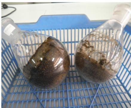
**Figure 3.** The evaporation results after tea material soaking with A) acetone and B) n-hexane (for interpretation of the references to color in the figure, the reader is referred to the web version of the articles).
