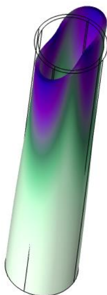
Figure 4. General form of loss of stability
