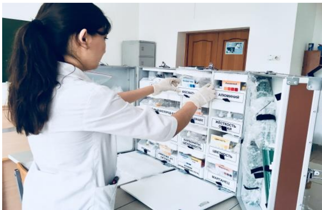
Figure 1. The study of the hydrochemical regime of water was carried out using the NKV-12 Express laboratory
