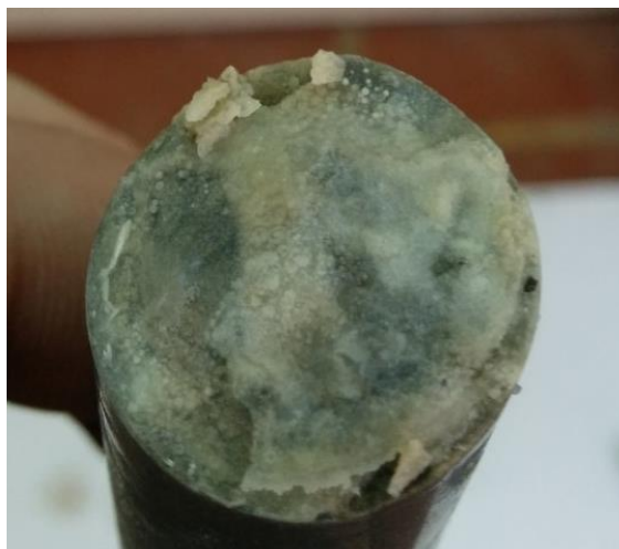
Figure 8. Crystal formation of magnesium chloride on a stone surface
