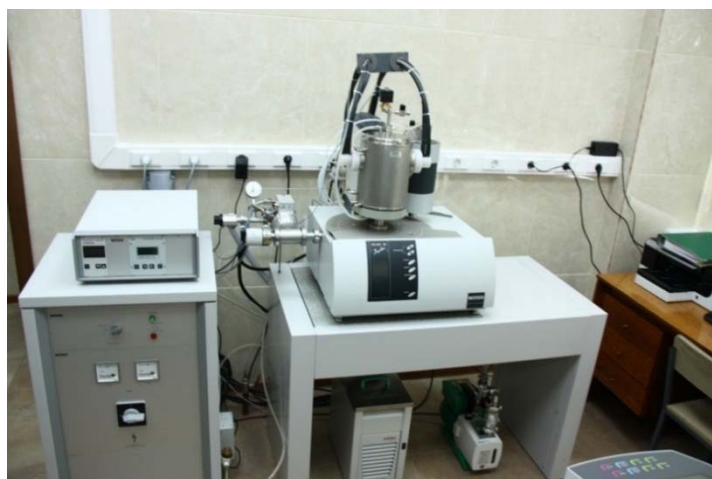
Figure 3. STA 449 F3 Jupiter device from NETZSCH (Germany)
