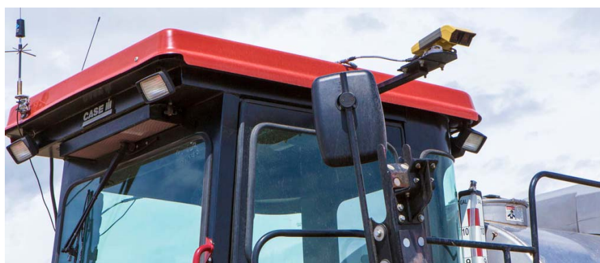
Figure 2. Tractor roof with CropSpecTM vegetation level sensor mounted on it
