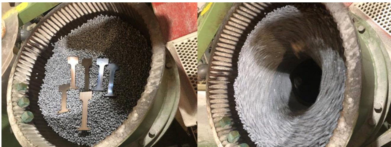
Figure 9. Installation for centrifugal hardening treatment (Rosler)
