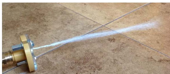
Figure 15. Experimental prototype of the switch-gear equipped with the indicator thread ("ponytail") when the air flows through the outlet channel for the conditions when the angle " \alpha " is equal to zero degrees
