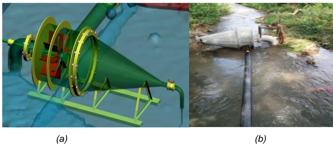
Figure 11. Types of an experimental model of a cylinder-conical version of a hydrocyclone of a micro HPP. a) type of test piece; b) the type of work of the sample in the river.
