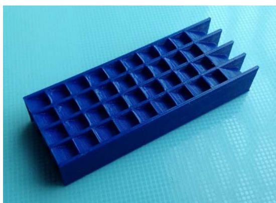
Figure 8. Experimental prototype of the mesh vane manufactured on a 3D printer for investigation of impeller machines with the mesh structure of channels
