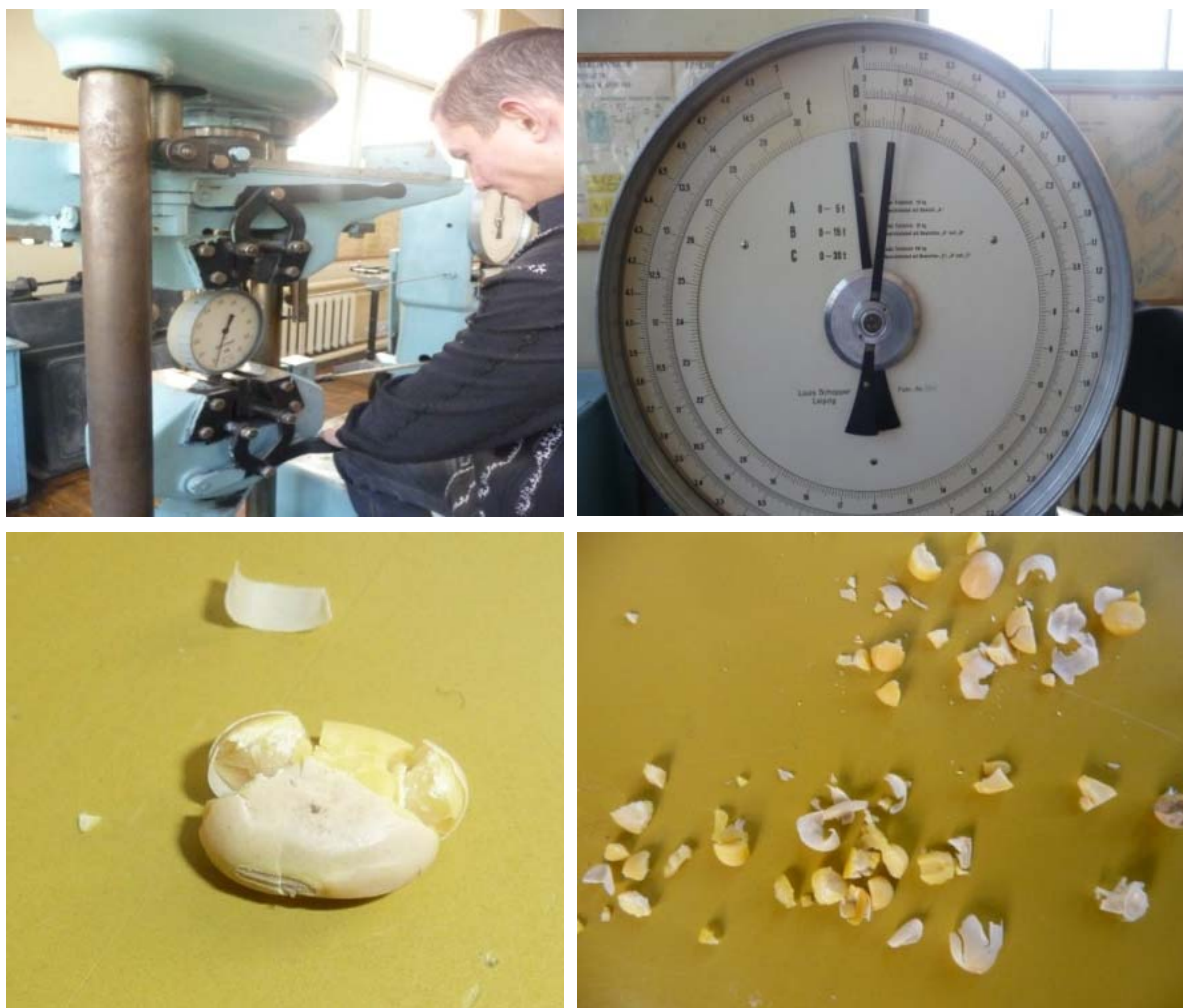
Figure 5. The relationship of the destruction of the swollen grains by means of pressure being applied
